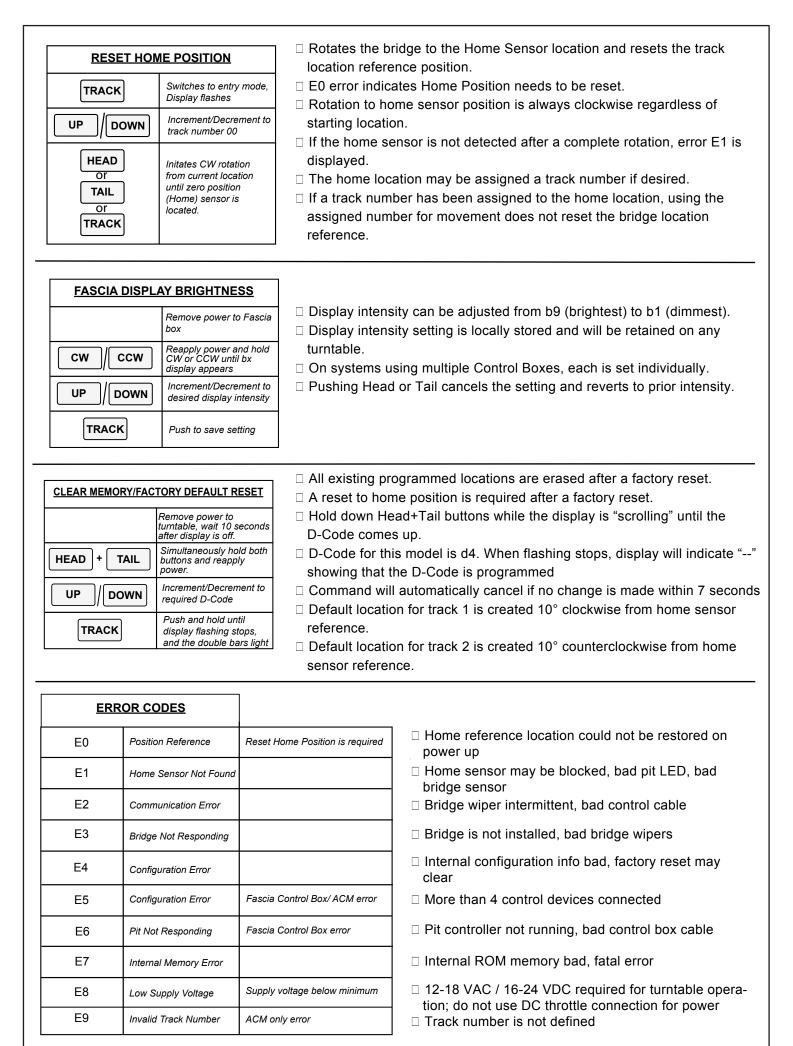
E0 Position Error can be cleared by pushing any key. Service track locations will not be correct until a reset of the home position is done. Other errors will clear automatically when the cause is corrected.
