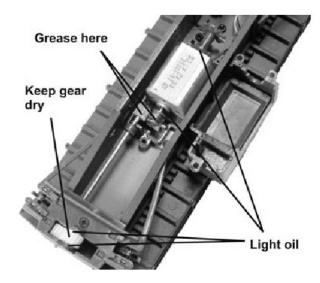
Apply a small drop of light oil for electric motors to the bearings; apply a light gear lubricant to the gear train as shown.
