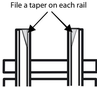
All service tracks must radially align with the bridge rails in a straight line with the track centerline aligned with the turntable center at the edge of the pit. You can use the bridge as a guide and sight along the rails to ensure a smooth transition from the bridge rails to the service tracks. Kinks in the rail
