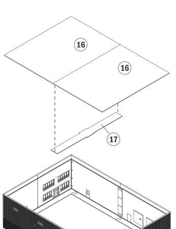
12. Place the two roof halves (16) upside down on a flat surface, and abut them so the edges with the raised alignment ridges are toward the center. Align roof connector (17) between the raised alignment ridges; glue where parts meet and allow to dry. Flip roof assembly over so the side with the roof connector (17) is facing downward.
