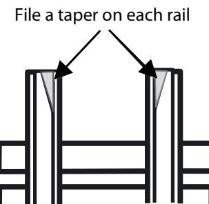
All service tracks must radially align with the bridge rails in a straight line with the track centerline aligned with the turntable center at the edge of the pit. You can use the bridge as a guide and sight along the rails to ensure a smooth transition from the bridge rails to the service tracks. Kinks in the rail
