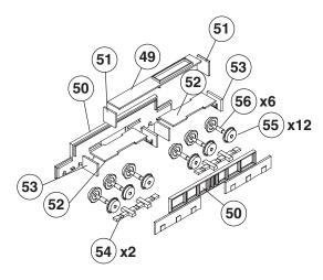
7. Glue the bogey top (49) and the lower tops (52) to one of the bogey sides (50). Next glue on the other side (50). Glue on the ends (51, 53). Glue the wheels (55) to the ends of the axles (56). Note: Push the wheel on until it stops. Set, do not glue, the axles into the slots on the insides of #50. Glue the wheel retainer (54) in place, making sure not to get any glue on the axles. Repeat this procedure three more times. Set aside.
