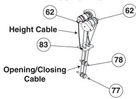
22. BUCKET HEIGHT CABLE: Cut a piece of string (length is dependent on how high or low you desire to hang the bucket) and tie a knot at one end and run it through the end hole on part #83. Wrap it around one of the drums and proceed down to the other end hole on #83. Tie it off with a knot.
