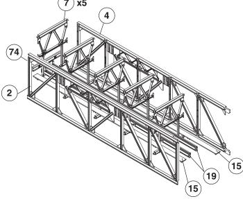
2. Glue the standard crossmembers (7) into the holes on the inside of the right rear truss (2). Glue the rear trolley rails (19) to the pegs on the inside of #7. Then glue the rear walkway sections (15) on both sides of the crossmembers. Next glue on the left rear truss (4). Glue on the end truss beam (74). Set aside.
