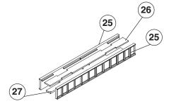
13. Glue the pier leg boxes (25, 26, 27) together and then onto the bottom of the gussets shown in step 12, The Truss Side View. Note: The bottom of the front box must have the two slots facing forward while the box at the back must have the slots facing backward.
