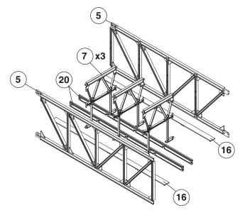
3. Glue the standard crossmembers (7) into the holes on the inside of the long middle truss (5). Note: For the medium option (B), use part #6. Glue the long middle trolley rails (20) to the pegs on the inside of #7 (for medium option, use part #21). Then glue the long middle walkways (16) on both sides of the crossmembers (use #17 for the medium option). Glue on the other long middle truss (5) (#6 for the medium option).
