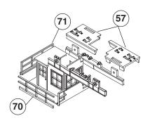
18. Glue the railings 70, 71 on. Place (do not glue at this time) the trolley floors (57) in position.
