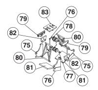
21. Place, do not glue, the bucket arm (80) into the holes in the bucket sides (75, 76) and then glue on the bucket bottom (81). Place the pegs on one side of the arms (80) into the holes in one of the upper sides (79). Also place the shaft of the upper pulleys (78) in the middle hole in part #79. Then push on the other upper side (79). Glue the top (83) on. Note: Do not get any glue on the arm pegs.
