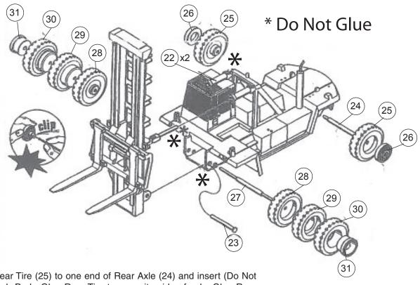
4) Glue a Rear Tire (25) to one end of Rear Axle (24) and insert (Do Not Glue!) through Body. Glue Rear Tire to opposite side of axle. Glue Rear Wheel Hubs (2x 26; one each side) to Rear Tires as shown.
