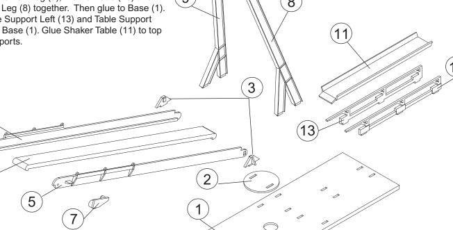
6. Glue the Frame Assembly and the Shaker Table Assembly to the base. There are Locator Holes in Base for easy assembly.
