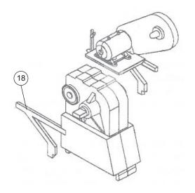
3. Glue the other bracket (18) into the notch in gearbox half #13. Then press fit the peg on bracket #19 into the hole in gearbox half #14 along with the horizontal brace into the notch in #14. NOTE: If you plan to motorize this kit do not glue this assembly in place.
