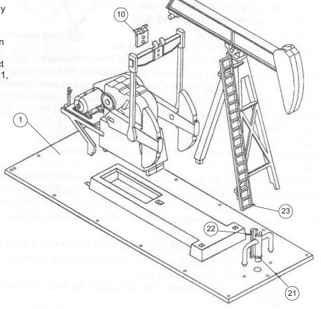
7. Cut a piece of wire 1 ½" long (3.7cm). On one end of the wire glue on the carrier bar (20) using CA type cement. Place the other end of the wire through the hole in the wellhead. NOTE: If you are motorizing this kit, bend the bottom of the wire into a small hook and
