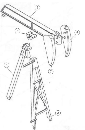
5. Glue the horse head sides (7, 8) to the walking beam (6), Glue the bearing (4), underneath the beam, in the middle. After that has dried completely, snap the top of the support brace (3) into the bearing. Then glue the support (2) to the brace.
