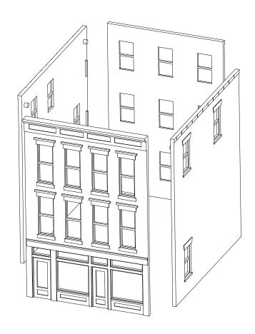
3) The acetate windows and printed interior graphics should be added now. Cut the acetate slightly larger than the window sizes and glue it in place using Walthers Goo® or other contact adhesive. Trim the individual art elements and tape them to the back of the clear glass using a quality tape. The roof can now be glued into position. Single or double stack chimneys are provided. Add as desired, or where shown, on the roof.
