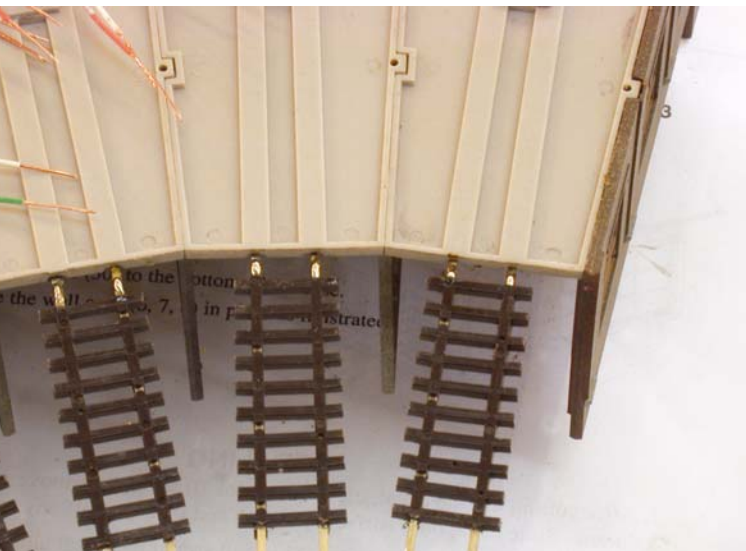
Left, power needs to be sent to the rails and I used the hidden wire method of attaching "downleads" to the bottoms of the rails. I placed them close to the foundation. I used alternating color pairs to help keep them separate as each will go to a separate momentary contact power switch. DCC users can run each pair to their bus lines. The turntable does not route power to those tracks. Right, I then drilled the holes for the roundhouse track wires.
