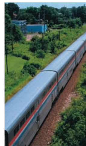
The eastbound Empire Builder is just a few hours from Chicago as it glides along the mighty Mississippi River at Savanna, IL in 1994. The train is detouring on BN because of a line closure on CP. Note the single weld line down the middle of the roof; Superliner II cars have a four panel roof.
